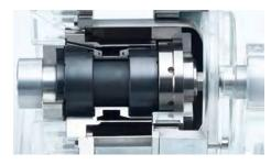
The pump power is transmitted from the drive shaft contact-free via the magnetic coupling. This ensures that the pump speed always corresponds to the drive speed. Thanks to the special bearings of the magnetic coupling's internal rotor, only the drive speed is transmitted to the drive shaft, avoiding any undesirable forces.
